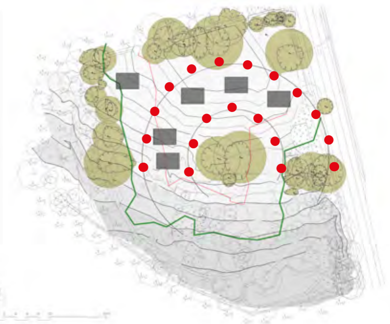
FIG 6. INITIAL DESIGN IDEA - CREATING A VIEWING ARC. BUILDINGS TO BE LOCATED WITHIN OPEN SPACE AREAS AND USING THE SITE TOPOGRAPHY TO ENHANCE AND PROTECT VIEWS OF THE WOODLAND
